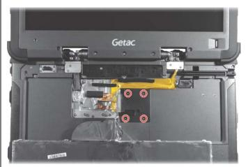
Screw P/N: 371102040610 (size: M2 x L6; torque: 2.0~2.5 kgf·cm)
