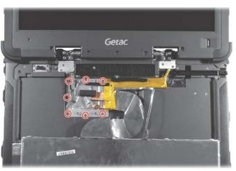
Screw P/N: 371102540510 (size: M2.5 x L5; torque: 3.0~3.5 kgf·cm)
