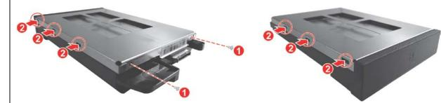
2. Detach the HDD from the HDD kit.
