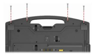
2. Turn S410 over and lay it down. Lift up the handle to detach it from S410. Two small covers will also come off.
