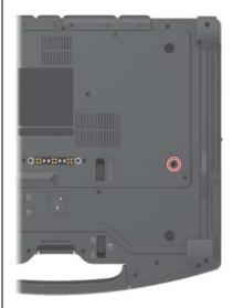
2. Slide the latch to the unlocked position ( ) ( ) and, while holding it there, pull the ODD kit out of the bay ( ).
