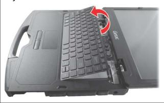
5. Open the Mylar film to access the connectors.
