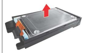
3. Disconnect the interface connector from the HDD.
